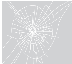
< Broken Laminated Glass >
