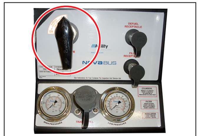
Figure 5 - Emergency Shut-Off Valve
