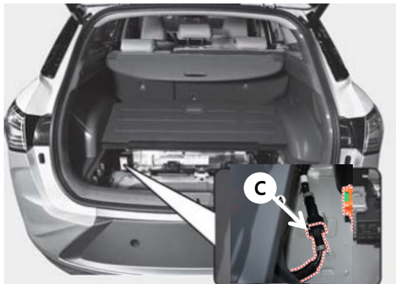
b. Disconnect the negative (-) 12 Volt battery cable connector (C) by pressing the connector tab and pulling apart
