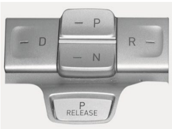
Step on brake pedal and Select(push) 'P' button on the shift selector console
