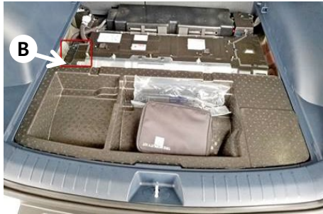
a. Remove the floorboard (A) and Styrofoam cargo tray (B) from the rear cargo area.
