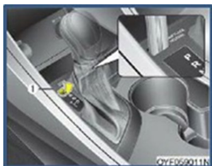
Step on brake pedal to park the vehicle, then position the shift lever in park (P)
