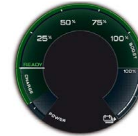
„READY“ Drive switched on Vehicle ready
