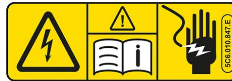
Examples of warning stickers in high-voltage vehicles.
